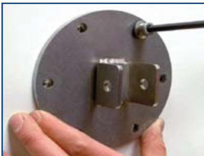
Secure the flange on the bearing side using the short M8 bolts with neoprene washers.
