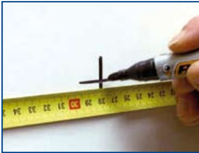
Mark the dimensions of the motor flange.
