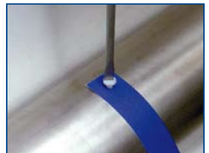
Attach the straps to the winding tube.
