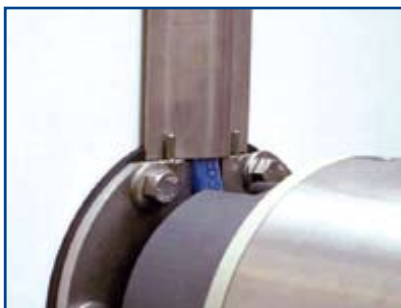
Slide the cable conduit behind the pins on the flange.
