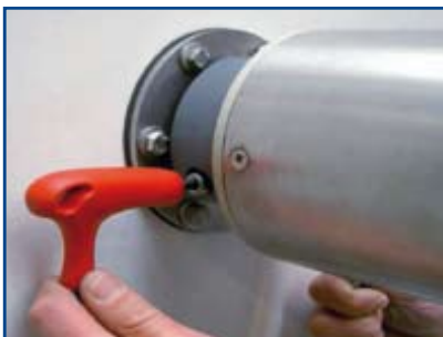
Secure the bolt with the crown nut.
