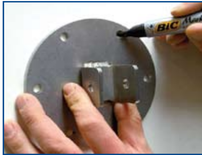
Place the bearing flange and mark the holes.
