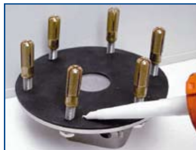
First thread the WAKO plugs onto the bolts (with neoprene washers), then apply sealant to the seal.
