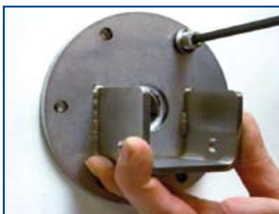
Secure the motor flange using the short M8 bolts with neoprene washers.
