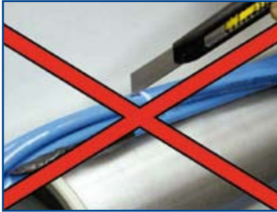
Do not cut the control cable loose with a blade.
