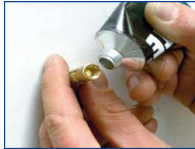
TIP! A bit of grease inside of the WAKO plug prevents the entry of dust that makes the bolts difficult to turn.
