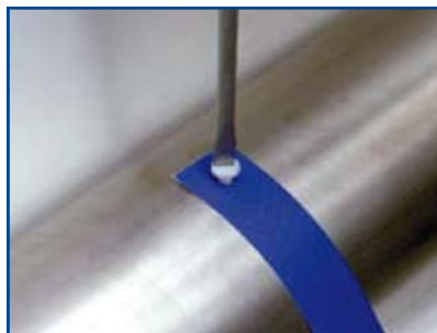
Attach the straps to the winding tube.
