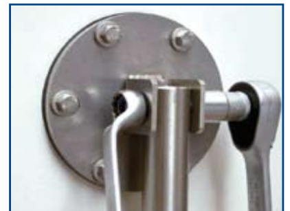
Attach the bearing shaft with bolt and self-locking nut.
